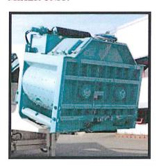
Twin horizontal shaft Mixer 3750/2500, for Voyager 90, with production capacity of 90m3/h, 3750lt ability of dry loading, 2500lt capacity in vibrated concrete. Also included is an automatic greaser, a 1,5 KW unloading hydraulic engine, two (2) 45Kw motors, surrounding visiting-working platform.
